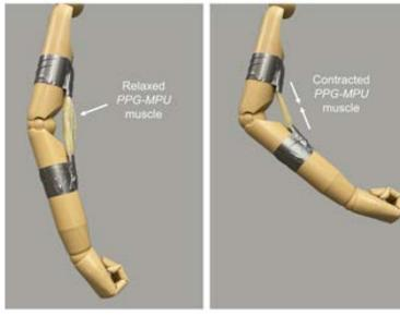
An artificial muscle made of a stretched shape memory polymer contracts upon heating, bending a mannequin's arm. Credit: Adapted from ACS Central Science 2021, DOI: 10.1021/acscentsci.1c00829
